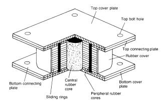
Fig. 3a Cross-section of R-FBI system
